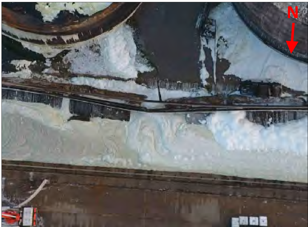
Photo 6: Closeup from aerial view of containment wall failure 14
