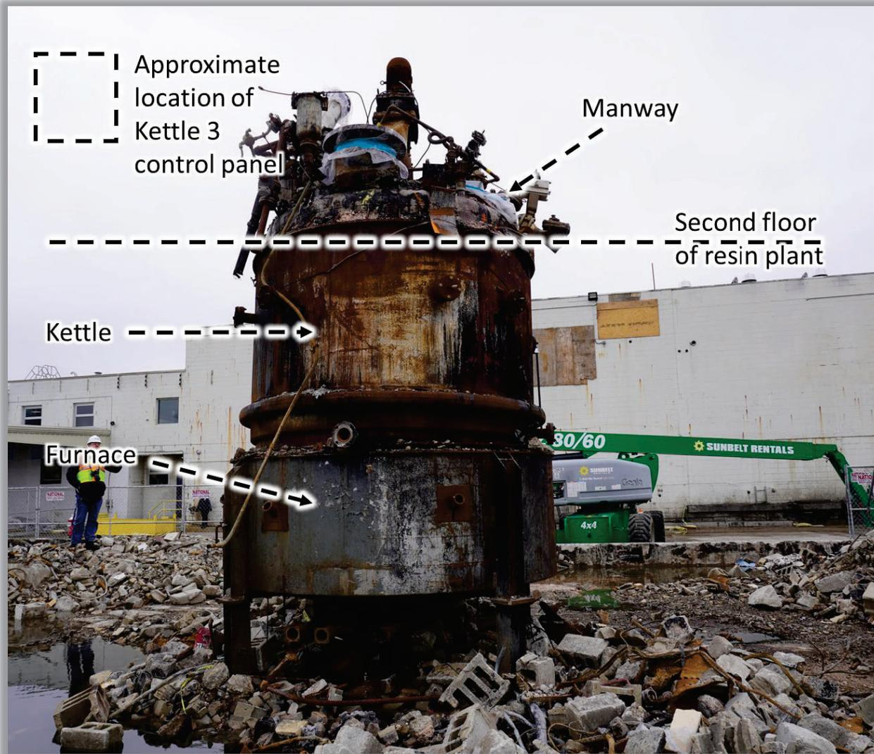
Figure 4. Photo of Kettle 3 during demolition. (Credit: CSB)
