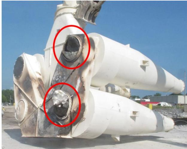
**Figure 55:** 4D Cyclones with rupture disks, with red circles indicating damaged rupture disks. (Credit: Didion, annotations by CSB)
