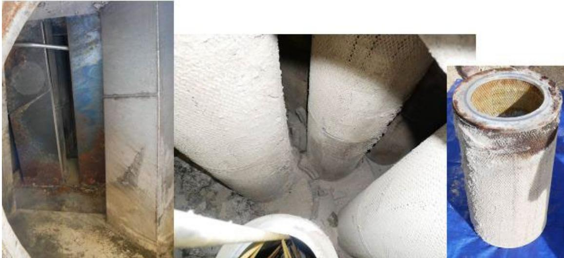
**Figure 39:** Torit Filter damage: inlet baffle heat damage (left), dark residue inside (center), and a filter element removed (right). (Credit: Didion)
