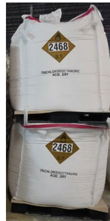
Figure 22. Super sacks storage method inside the Bio-Lab Conyers Plant 6. (Credit: CSB)
