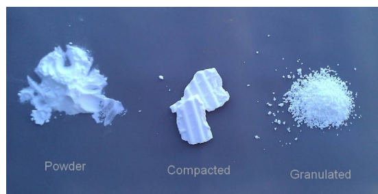
Figure 2. Forms of Bio-Lab's TCCA-based formulation. (Credit: Bio-Lab)
