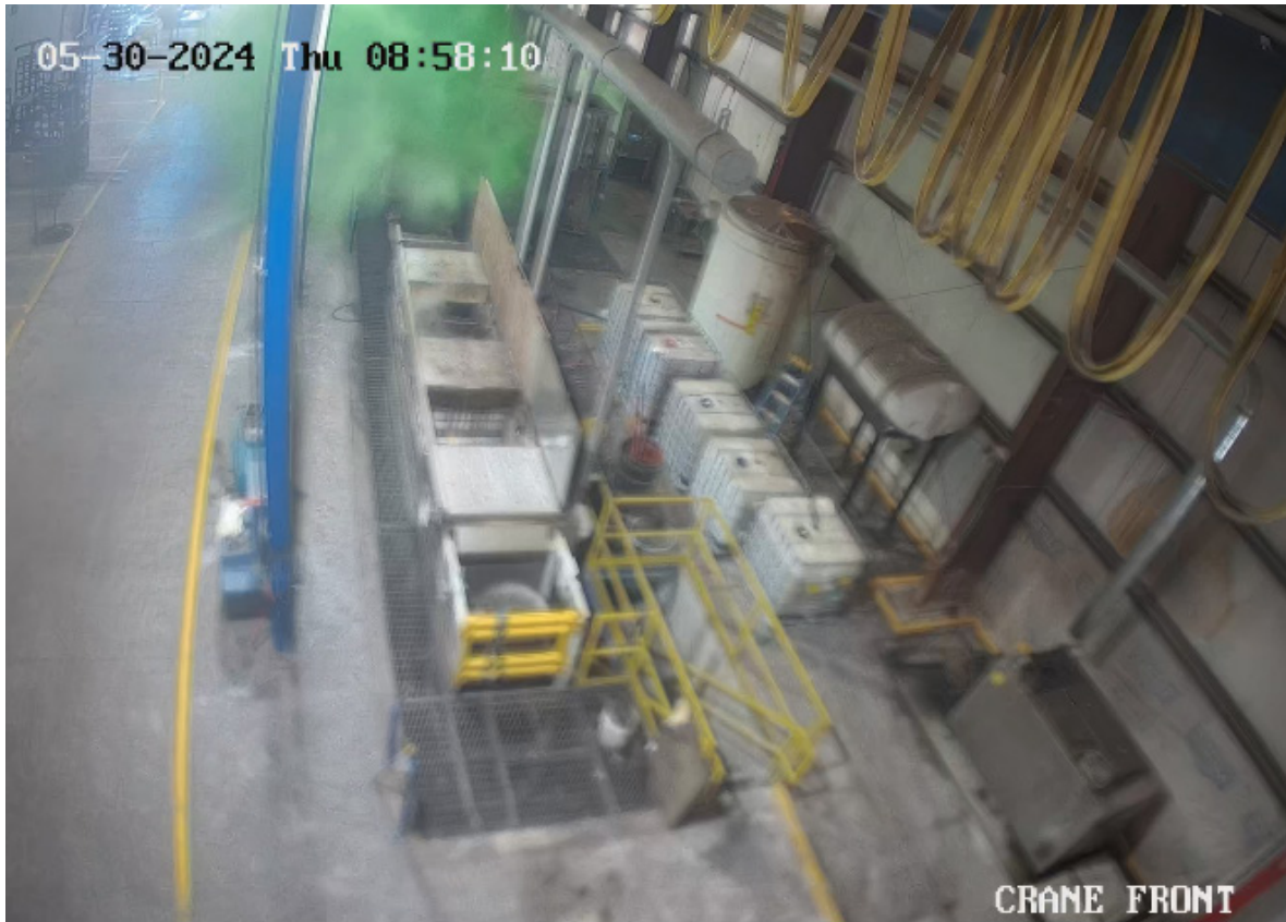
Figure 12. Molten oxidizing salt erupting from the oxidizing tank. (Credit: TS USA)
