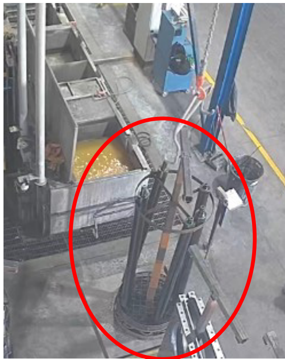
Figure 7. Five rollers are placed in the fixture. (Credit: TS USA, annotated by CSB)
