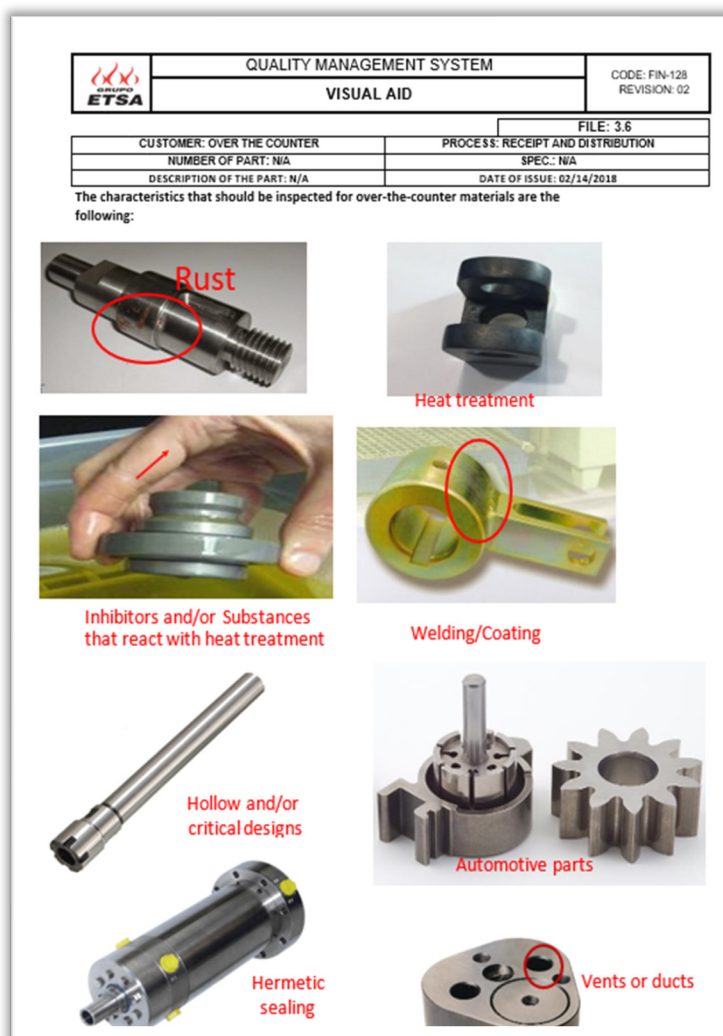
Figure 21. The visual aid created by TS ETSA for part inspections. (Credit: TS ETSA, translated by the CSB)
