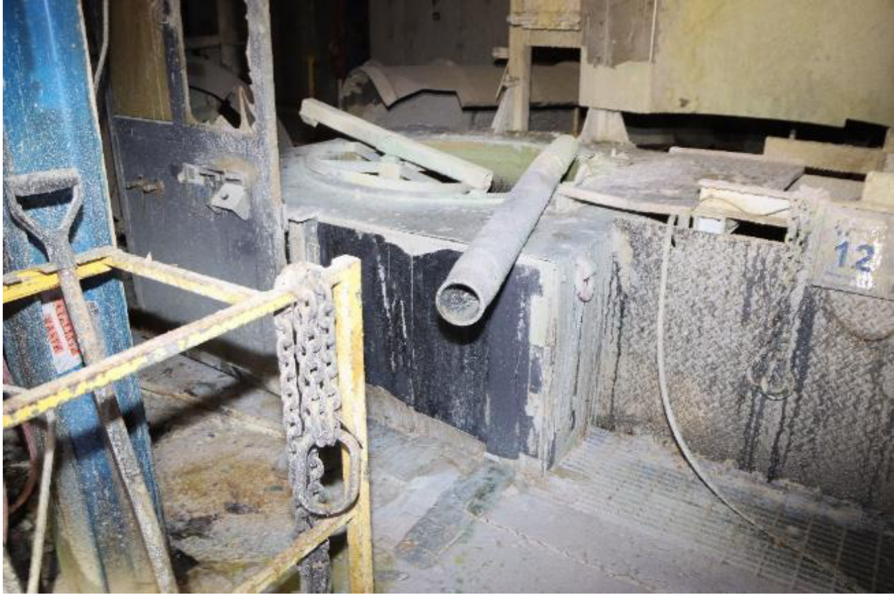
Figure 13. Roller in its final resting state following the explosion, with a missing press fit end. (Credit: TS USA)
