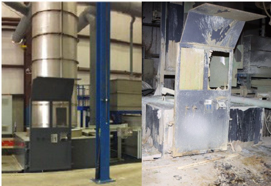
Figure 17. Protective barrier at the oxidizer bath, pre-incident (left) and post-incident (right). (Credit: TS USA)
